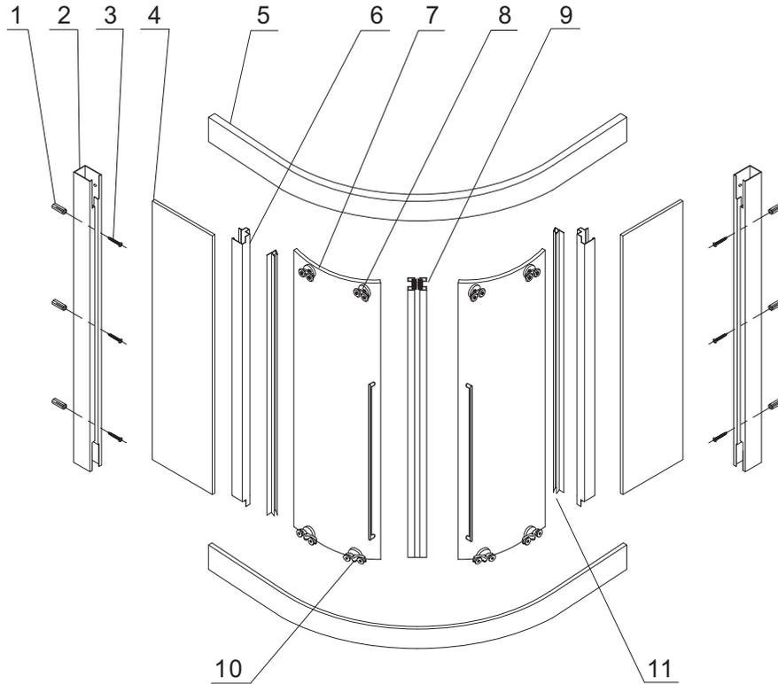
**7.** When installing the door magnets, ensure that the positioning is correct - the closed end should be at the bottom. Apply the clear silicone to the inner side of a door magnet strip. Fit it on the door glass one at a time from the bottom to the top. Carefully secure.
